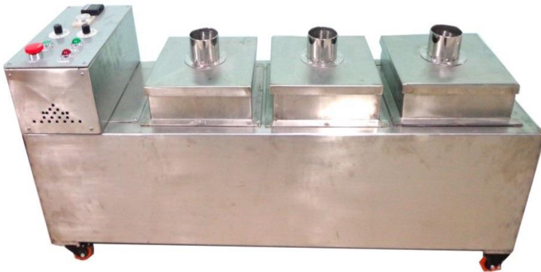
Sample Dryer- Simple is Effective Drying equipment with heated air (3 units) and drying temperature controlling system
