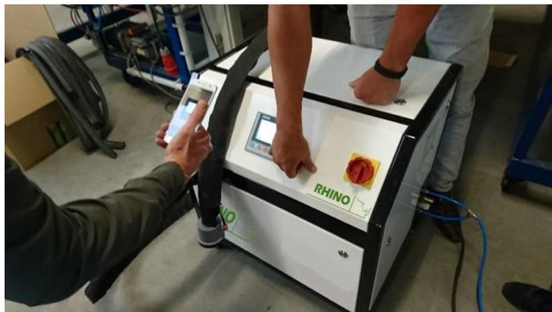
The new generation of our vacuum machines is of HS type. In combination with patented high speed valve, this machine offers an extremely quick and easy to use solution to vacuum pack large volumes. If required, you can flush the packaging with external gas for modified atmosphere packaging.
