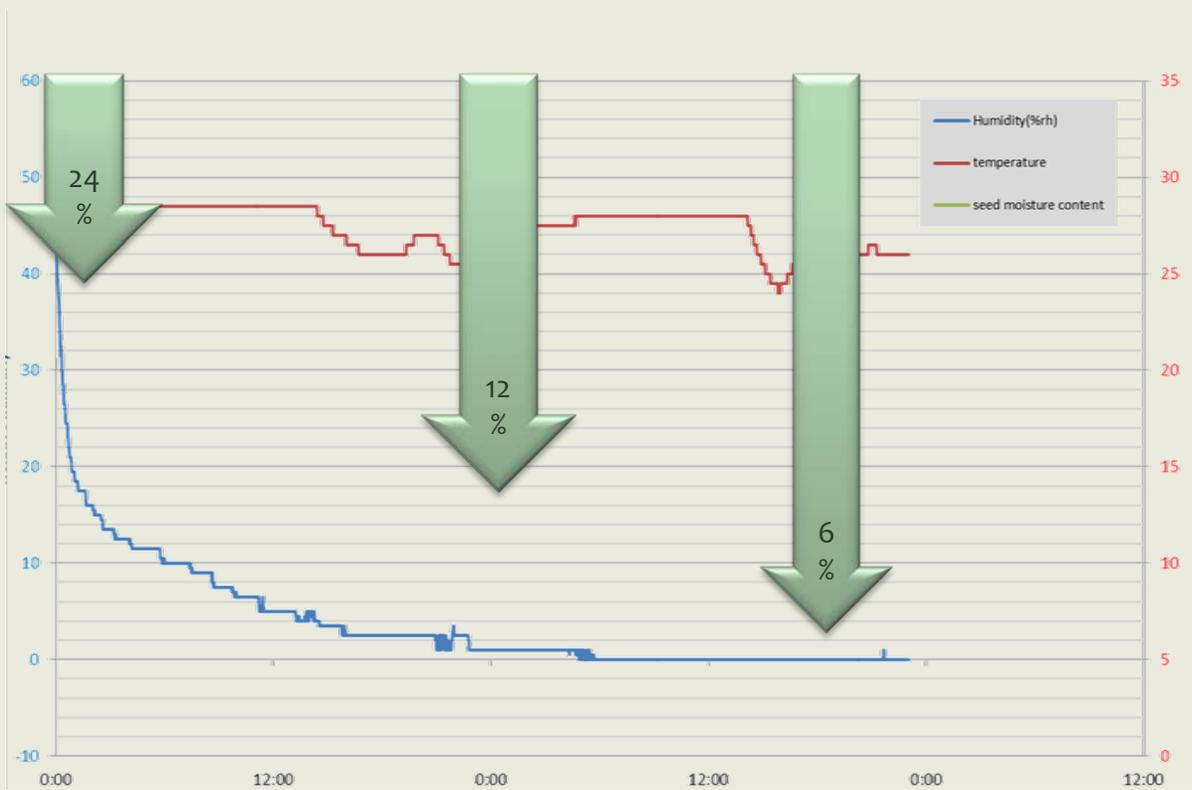
Temperature, RH and SMC during drying of a rice sample (48 Hours)
